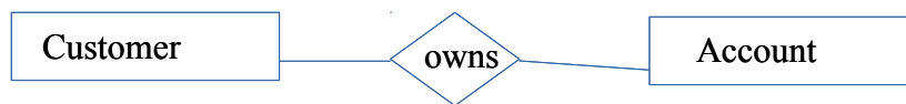
Figure 2 - ERD showing that a Customer entity class is related to an Account entity class via an owns relationship class
