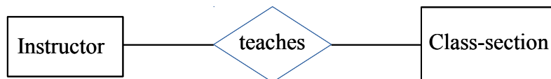
Figure 3 - ERD showing that an Instructor entity class is related to a Class-section entity class via a teaches relationship class
